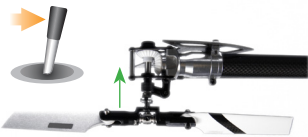
Use rudder stick to move the servo to the maximum allowed deflection
