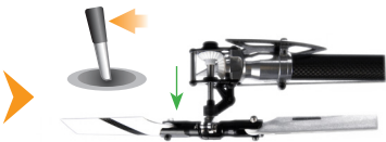
Use rudder stick to move the servo to the minimum allowed deflection
