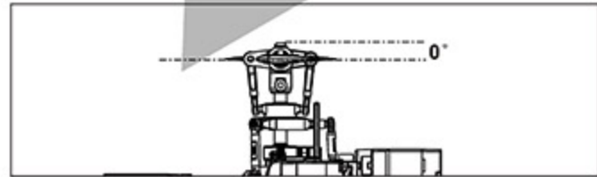
Stick position at middle/Throttle 85~90%/Pitch 0° 搖桿中速/油門85~90%/Pitch 0°
